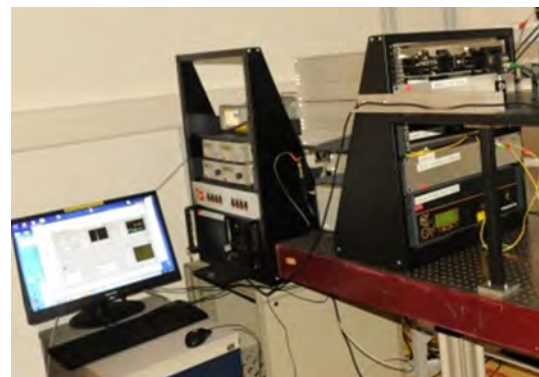
Fig. 4 The integrated engineering model of fiber laser HEPILAS for CO 2 monitoring from space.
